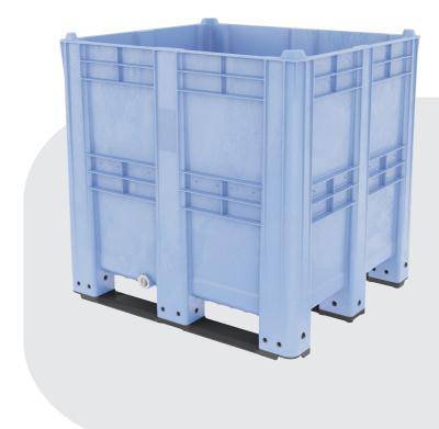
DOLAV Type 1120 box pallets have been the leading containers in Israel's agricultural market for over 40 years. The 700-litre box is made of four massive corner pillars and three long floor beams that give it unbeatable stacking and impact qualities. These box pallets incorporate our exclusive anti-slip corners that provide them with high stacking capacity of up to 8 boxes in cooling storage. The 1120 boxes are produced with UV protection suitable for increased long-term sun exposure.
